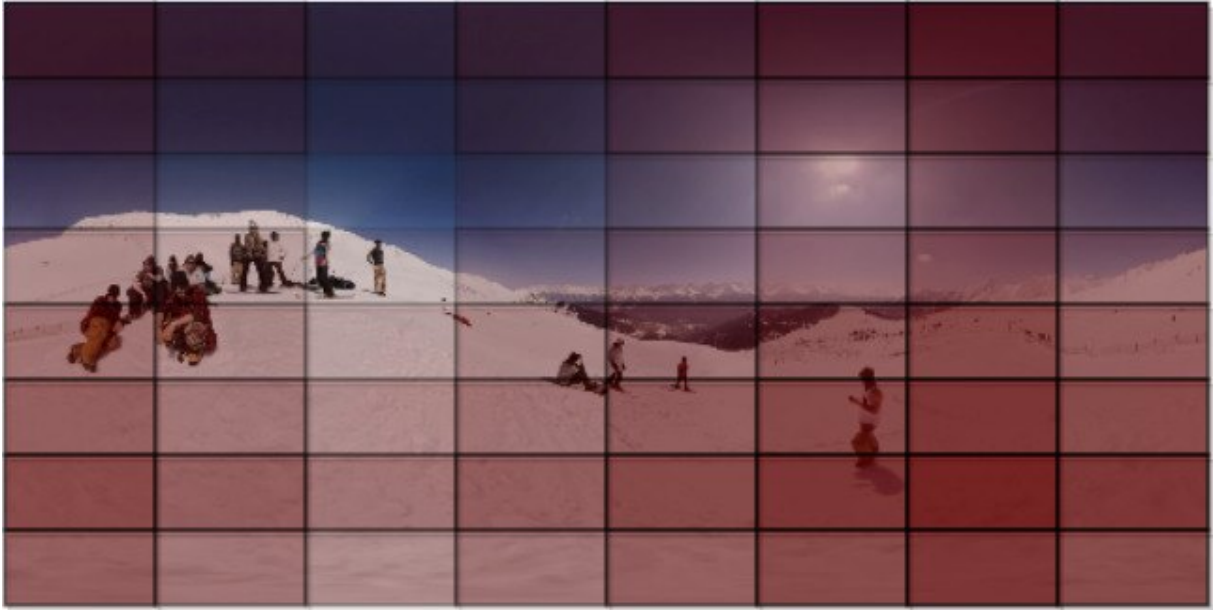
Figure 4.6: Pyramid Model of Bitrate Allocation. Consider tiles to be numbered as (x,y) , where x and y are the horizontal and vertical positions of the tile from the top-left corner. In this figure, An equirectangular frame split in 8 \times 8 tile format, which has viewport at tile (3,3) . Lower opacity signifies higher proportion of bitrate to be allotted to the tile
